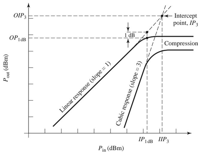
**FIGURE 10.17** Third-order intercept diagram for a nonlinear component.
