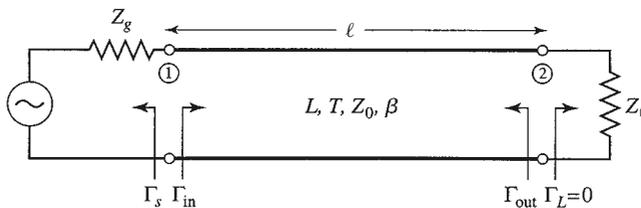
**FIGURE 10.12** A lossy transmission line at temperature  $T$  with an impedance mismatch at its input port.
