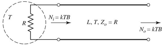
**FIGURE 10.8** Determining the noise figure of a lossy line or attenuator with loss  $L$  and temperature  $T$ .
