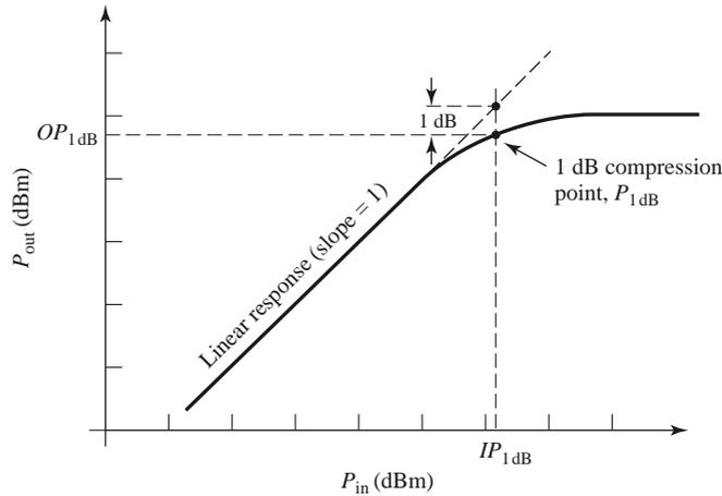
**FIGURE 10.15** Definition of the 1 dB compression point for a nonlinear amplifier.
