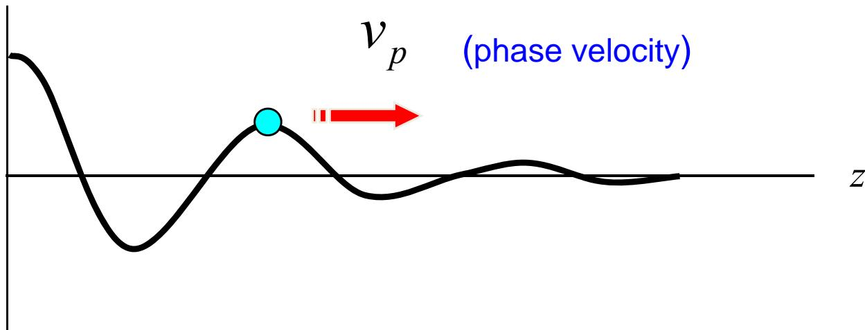
$$v^+(z, t) = |V_0^+| e^{-\alpha z} \cos(\omega t - \beta z + \phi)$$
