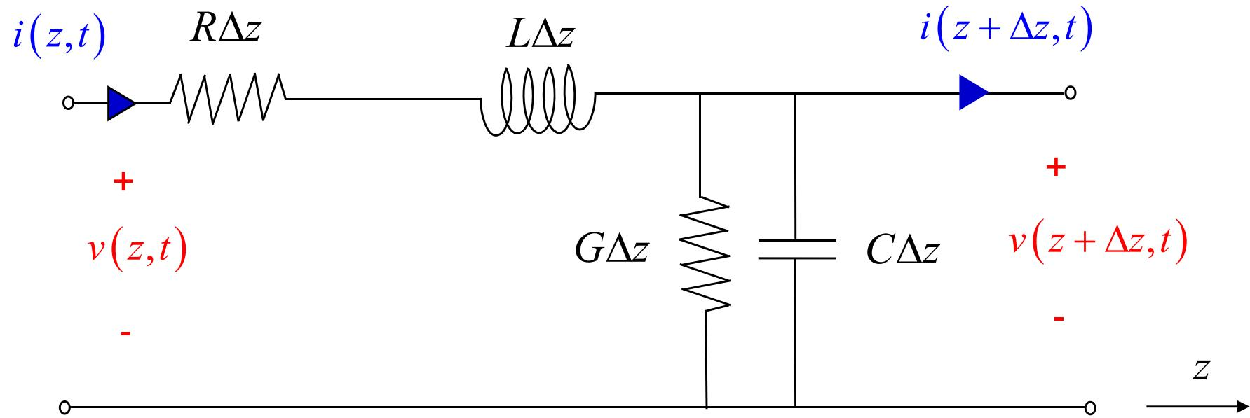
$$v(z, t) = v(z + \Delta z, t) + i(z, t)R\Delta z + L\Delta z \frac{\partial i(z, t)}{\partial t}$$
