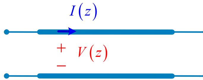
$$V(z) = V_0^+ e^{-\gamma z} + V_0^- e^{+\gamma z}$$
