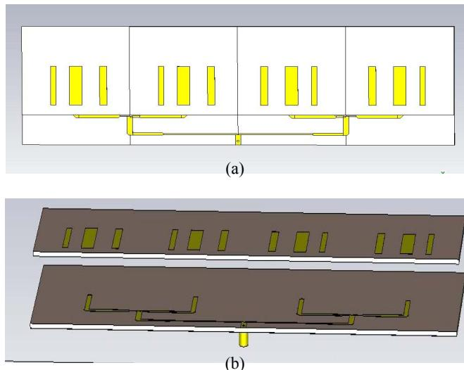
Fig 4. Antenna Design (a) top view (b) exploded view
