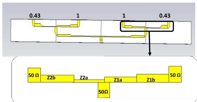
Fig 2. Unequal 4-way power divider
