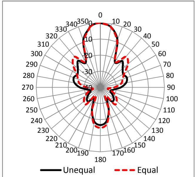
Fig 5. Radiation pattern at  $\phi = 0$
