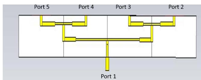
Fig 1. Equal 4-way power divider
