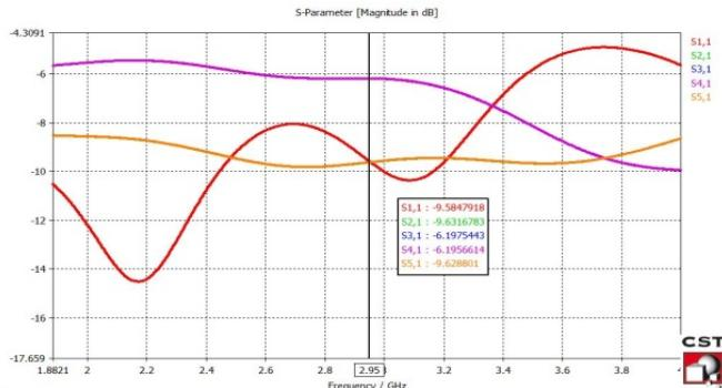
Fig 3. S-paramater simulation of unequal 4-way power divider
