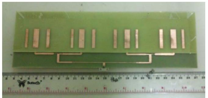
Fig 6. Photo of the fabricated antenna
