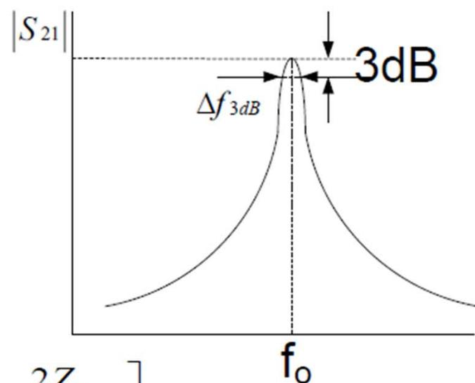
$$@ f_o : [Z] = \begin{bmatrix} R & R \\ R & R \end{bmatrix}, [S] = \begin{bmatrix} \frac{R}{R+2Z_o} & \frac{2Z_o}{R+2Z_o} \\ \frac{2Z_o}{R+2Z_o} & \frac{R}{R+2Z_o} \end{bmatrix} \dots \text{prob 4.11}$$
