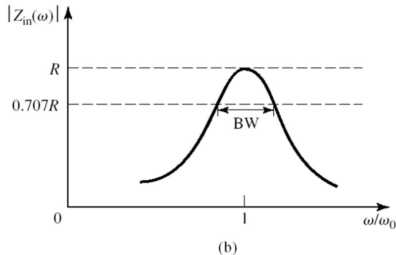
A parallel RLC resonator and its response. (a) The parallel RLC circuit. (b) The input impedance magnitude versus frequency.
