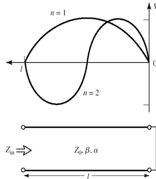
A short-circuited length of lossy transmission line and the voltage
