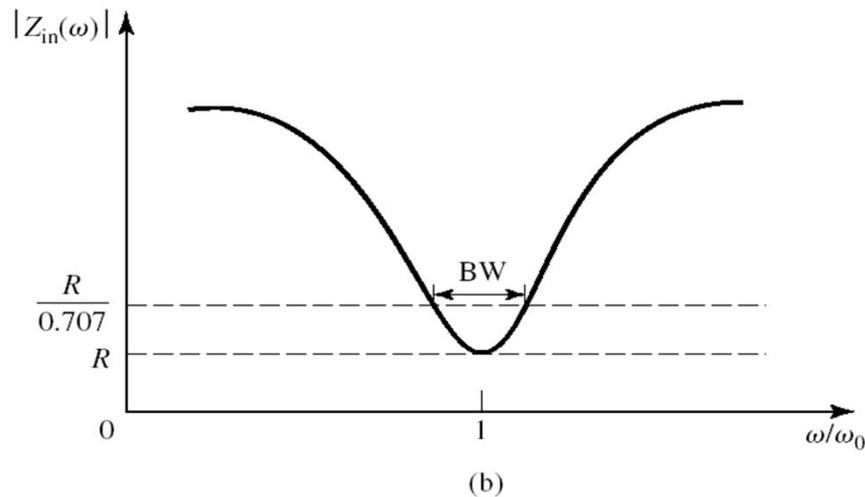
A series *RLC* resonator and its response. (a) The series *RLC* circuit. (b) The input impedance magnitude versus frequency.
