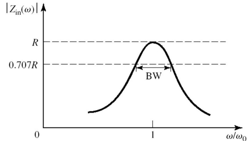
The input impedance magnitude versus frequency.
