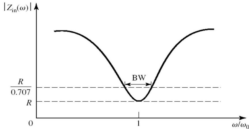
The input impedance magnitude versus frequency.
