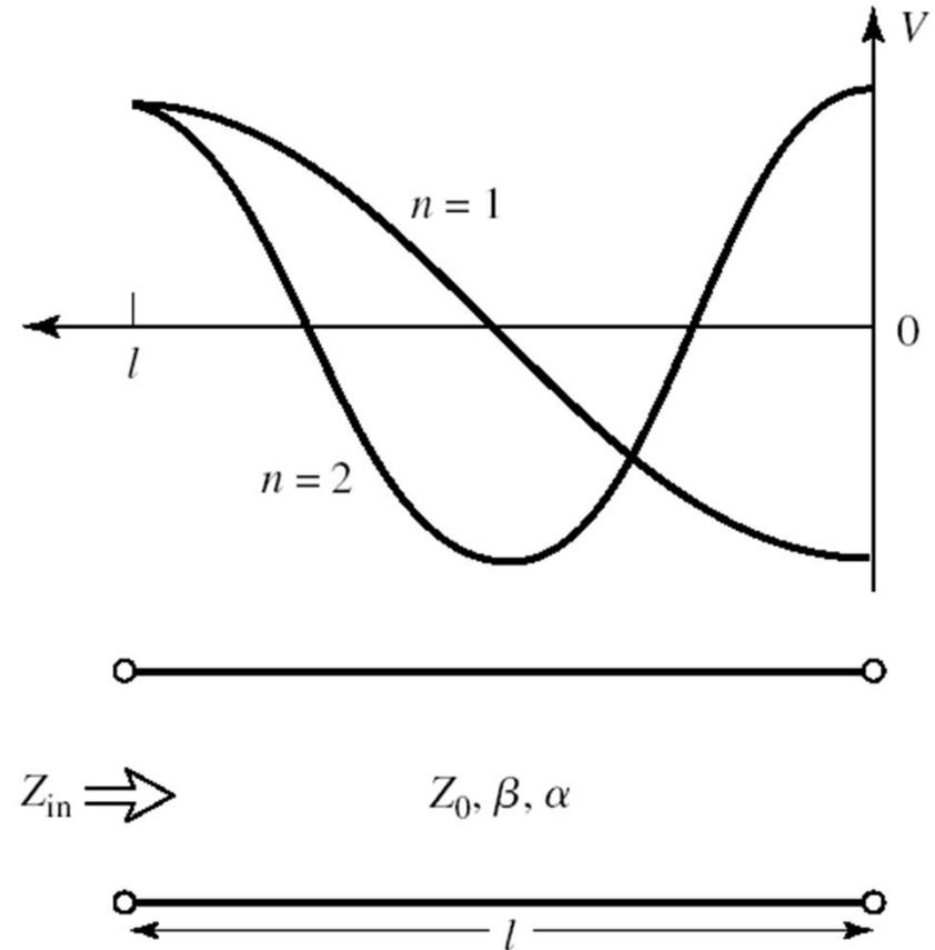
An open-circuited length of lossy transmission line, and the voltage distributions for  $n = 1$  resonators.
