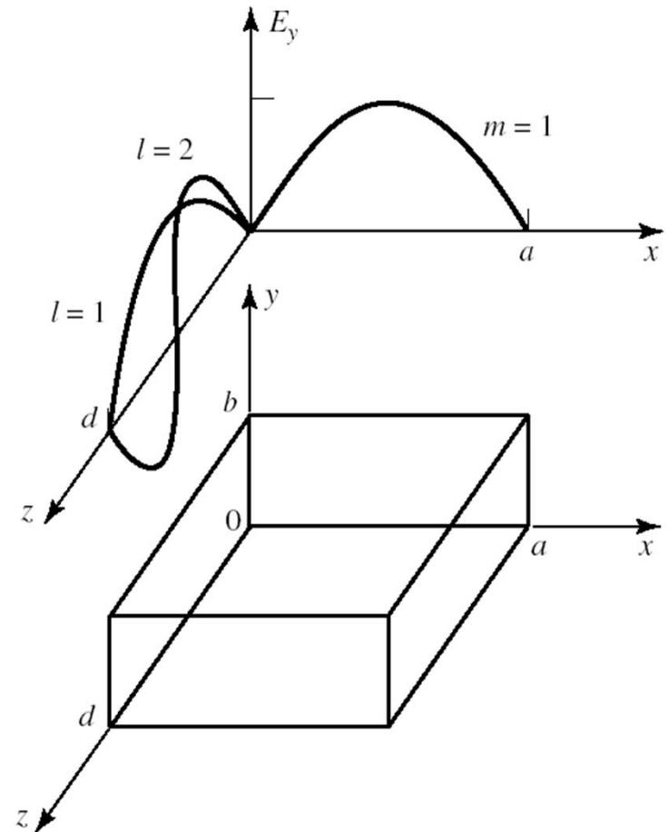
A rectangular resonant cavity, and the electric field distributions for the TE<sub>101</sub> and TE<sub>102</sub> resonant modes.
