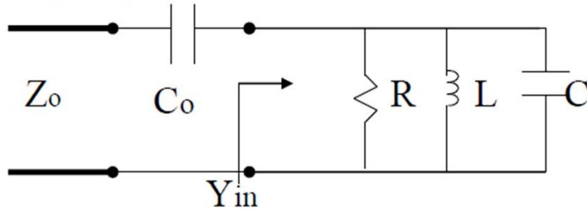
$$R=1000\ \Omega, L=1.26\text{nH}, \\ C=0.804\text{pF}, Z_o=50\ \Omega$$
