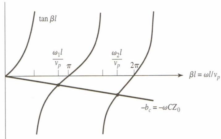
Solutions to (6.78) for the resonant frequencies of the gap-coupled microstrip resonator.
