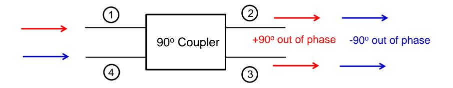
■The signal from port 1 splits evenly between ports 2 and 3, with a 90° phase difference.
