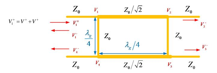
$$S_{31} = \frac{V_3^{-}}{V_1^{+}} \Big|_{a_2 = a_3 = a_4 = 0} \implies S_{31} = \frac{V_3^{-e} + V_3^{-o}}{V^{+} + V^{+}} = \frac{V_3^{-e} + V_3^{-o}}{2V^{+}} = \frac{V_2^{-e} - V_2^{-o}}{2V^{+}} = \frac{1}{2} \left( S_{21}^e - S_{21}^o \right) = \frac{1}{2} \left[ \left( \frac{-1 - j}{\sqrt{2}} \right) - \left( \frac{1 - j}{\sqrt{2}} \right) \right] = \frac{-1}{\sqrt{2}}$$
