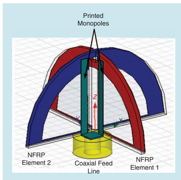
**FIGURE 11.** The 3-D view of a GPS L1 CP antenna with two orthogonally oriented NFRP elements [69].
