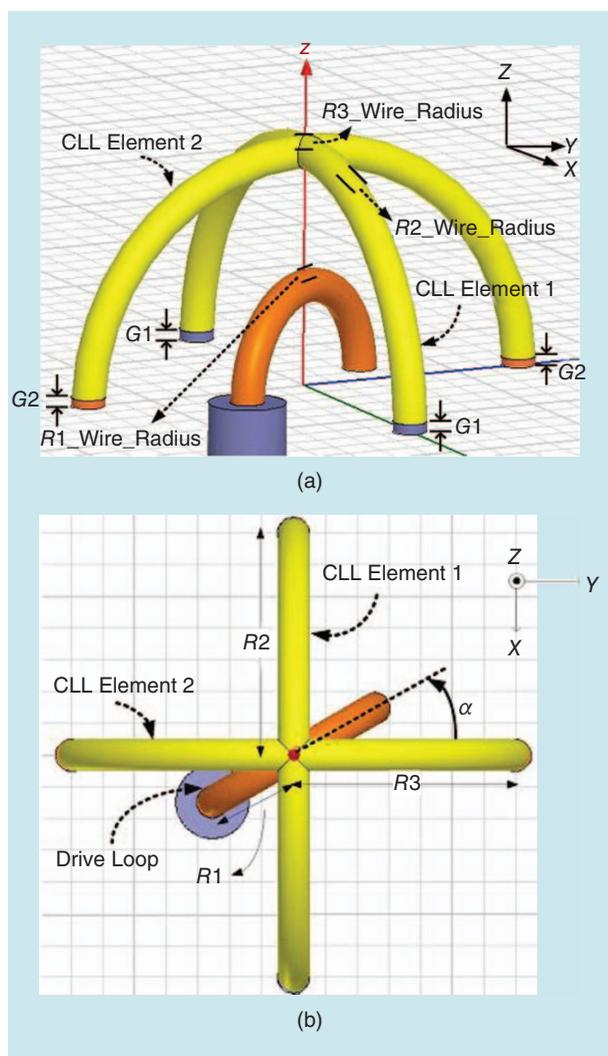
**FIGURE 10.** A GPS L1 CP NFRP wire antenna [68]. (a) The 3-D view. (b) The top view.  $R1 = 5.9 \text{ mm}$ ,  $R1\_wire\_radius = 1.0 \text{ mm}$ ,  $R2 = R3 = 14.0 \text{ mm}$ ,  $R2\_wire\_radius = R3\_wire\_radius = 1.0 \text{ mm}$ ,  $G1 = 0.193 \text{ mm}$ ,  $G2 = 0.182 \text{ mm}$ , and  $\alpha = 30^\circ$ .
