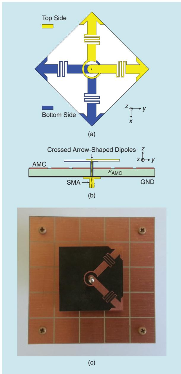
**FIGURE 19.** The low-profile CP crossed dipole integrated with a finite AMC surface for dual-band operation [79]. (a) A single-band radiator. (b) A cross-sectional view. (c) The top view of the fabricated prototype. SMA: subminiature version A. (Photo courtesy of Taylor & Francis.)
