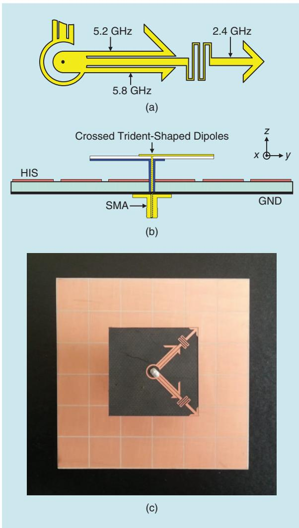
**FIGURE 20.** A CP crossed dipole antenna for 2.4-/5.2-/5.8-GHz WLAN applications [80]. (a) Trident-shaped dipole arm and vacant-quarter printed ring. (b) Cross-sectional view. (c) Top view of the fabricated prototype. SMA: subminiature version A.
