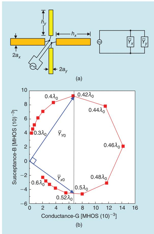
**FIGURE 8.** The two orthogonal cylindrical dipoles fed in parallel. (a) The arrangement of the dipoles and its equivalent circuit [52]. (b) The input admittance of a single dipole as a function of its length.
