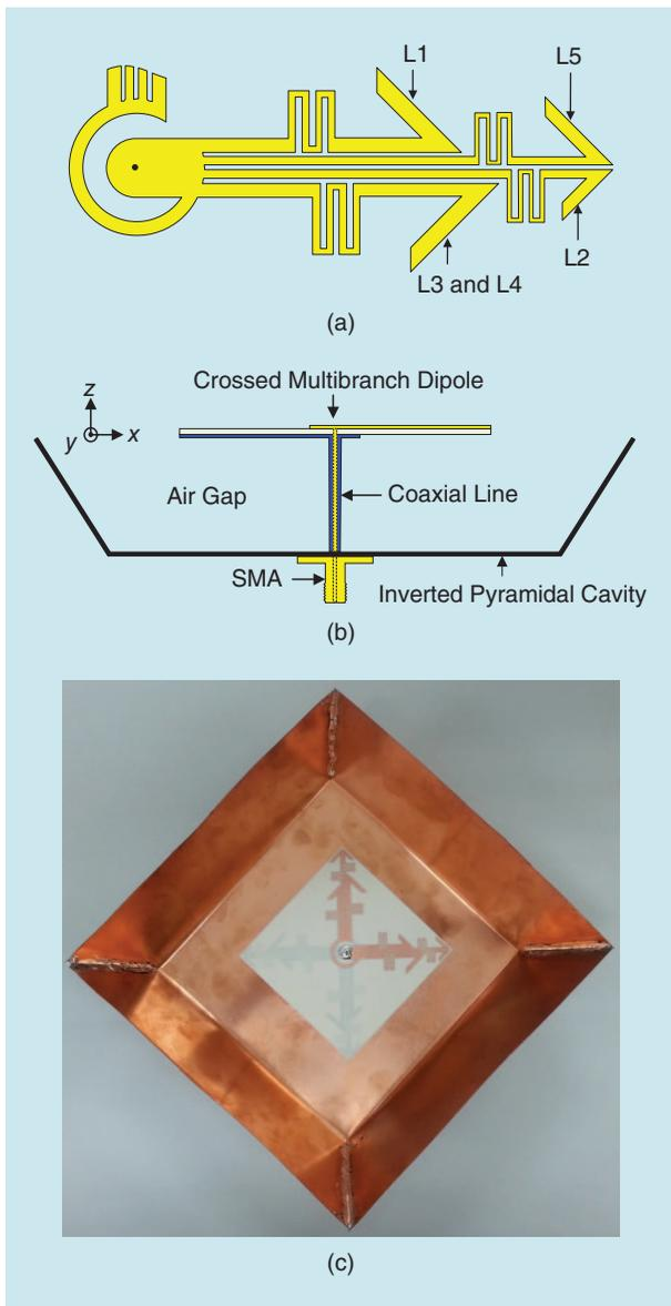
**FIGURE 18.** A multiband CP, crossed dipole antenna for GPS L1–L5 bands [78]. (a) The multibranch dipole arm and vacant-quarter printed ring. (b) A cross-sectional view. (c) The top view of the fabricated prototype. SMA: subminiature version A.
