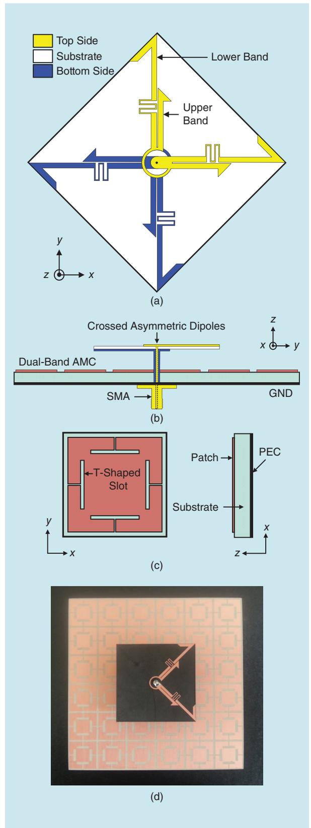
**FIGURE 21.** A CP crossed asymmetric dipole antenna integrated with a dual-band AMC surface [81]. (a) Radiator. (b) Cross-sectional view. (c) Unit cell of the dual-band AMC. (d) Top view of the fabricated prototype. SMA: subminiature version A.
