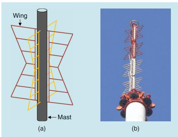
**FIGURE 3.** A batwing antenna. (a) The normal configuration [4] and (b) a superturnstile television broadcasting antenna at the Muehlacker television transmitter, Muehlacker, Germany. [Source: Figure 3(b) is from Wikipedia, the free encyclopedia. [https://en.wikipedia.org/wiki/Batwing\\_antenna](https://en.wikipedia.org/wiki/Batwing_antenna).]
