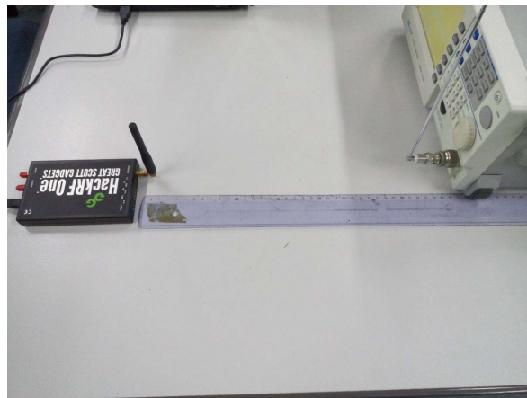
Fig. 2. HackRF One measuring RF signals compared to traditional spectrum analyzer.
