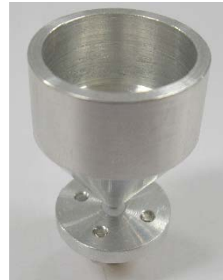
Fig. 11. Fabricated conical-cylindrical monopole antenna.
